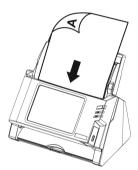
2. If you need to scan long documents, pull out the paper feeder extension and stacker to support scanned documents.
